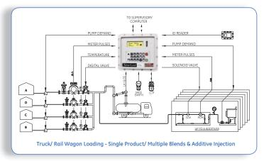
Directly interfaces with flow meters, digital control valves, additive injector panels, safety interlocks and Remote Interaction Terminal (RIT)
